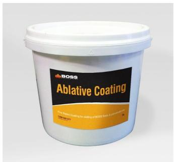
Ablative Coating has been developed to seal Bulkhead Batts once installed in aperture. Once the ablative coating is applied it prevents the passage of fire and smoke between fire rated compartments giving up to FRL -/240/180 with BOSS Batts to AS1530.4:2014 and AS4072.1-2005.
