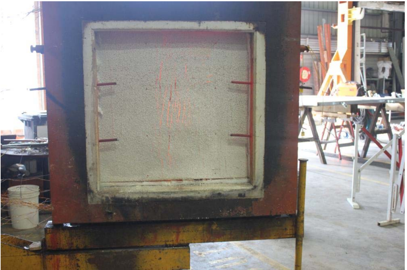
PHOTOGRAPH 13 –EXPOSED FACE OF SPECIMENS AFTER THE CONCLUSION OF TESTING
