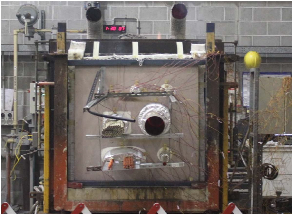
PHOTOGRAPH 6 – SPECIMENS AT THE CONCLUSION OF TESTING - 90 MINUTES
