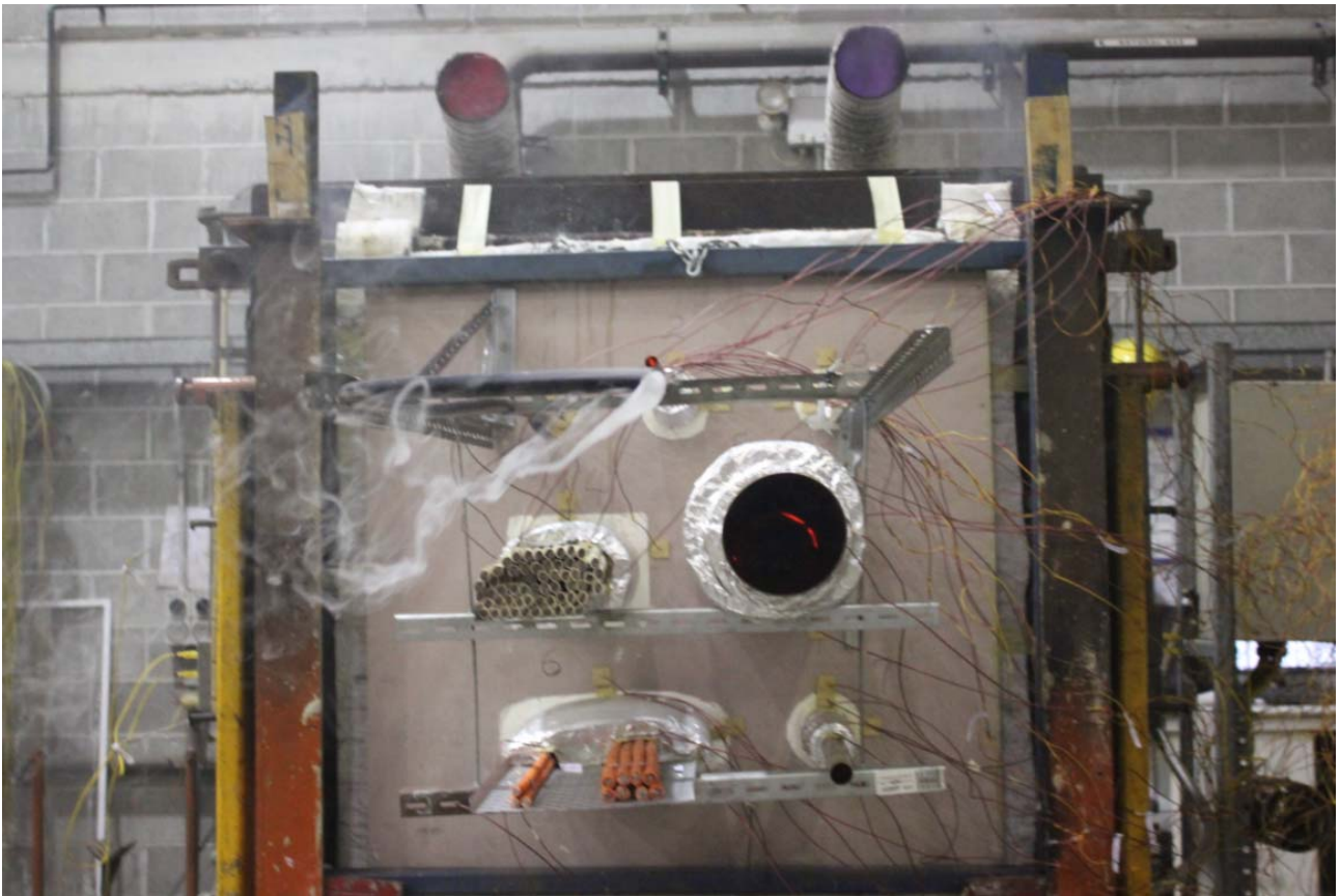
PHOTOGRAPH 5 – SPECIMENS AFTER 60 MINUTES OF TESTING
