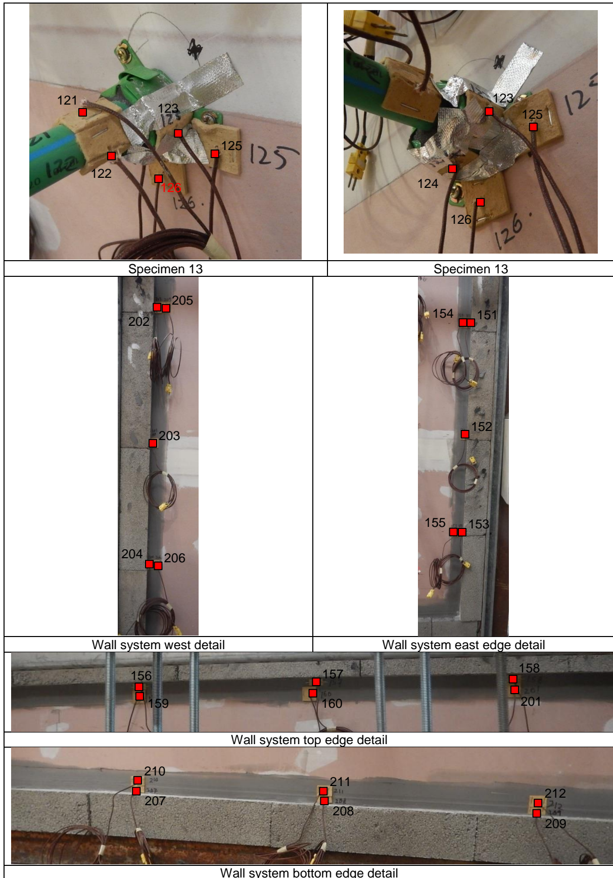
Figure A4.1: Unexposed surface thermocouple locations
