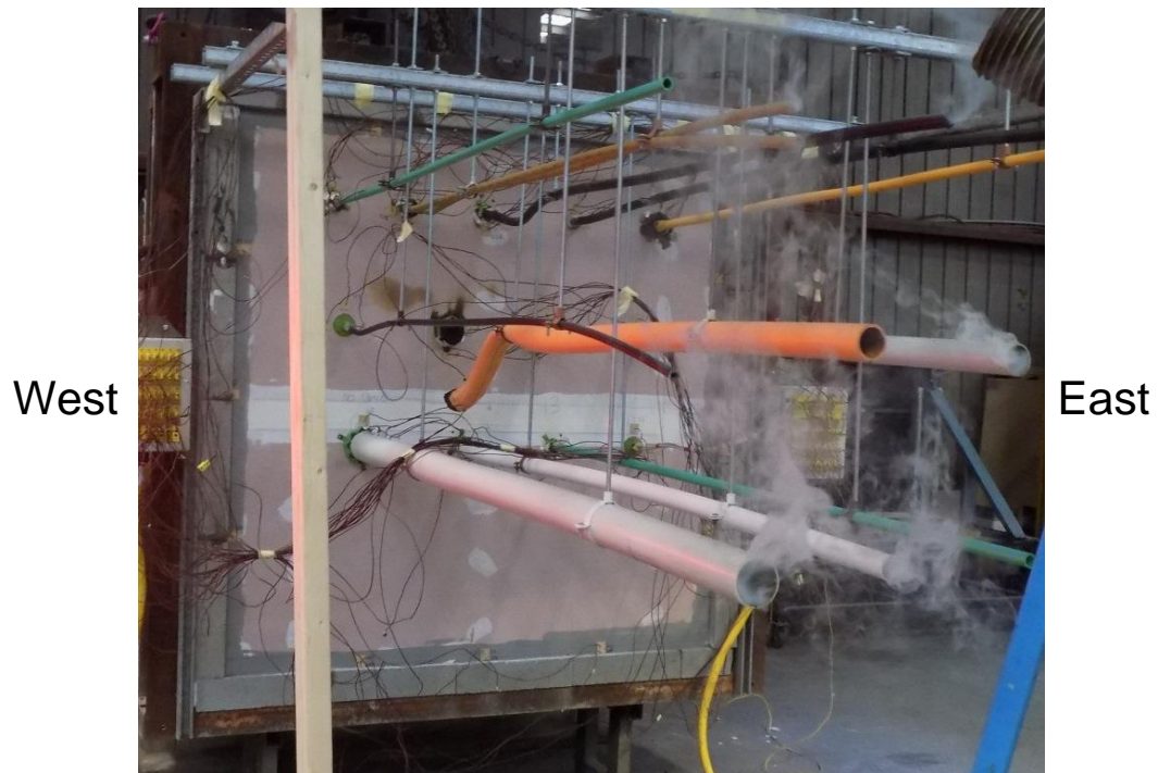
Figure A6.3: Unexposed face of specimen at the end of the test.
