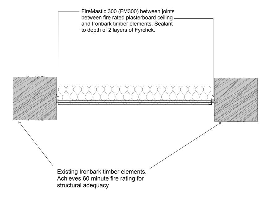
Ceiling support system including furring channels and hangers as specified.
